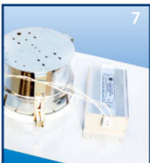
Completed ballast connection
